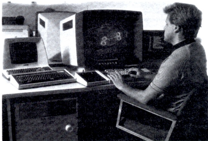
The technical directing of the action in computer simulated scenes is done first in vector form on a previewing system supplied by Interactive Machines, Inc.
